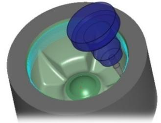
**Parallel Cut Surface Machining**
