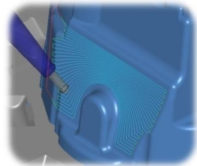
The options available may change depending on the type of 5-axis toolpath. In the linking the user can control the entry / exit moves and the transition.
