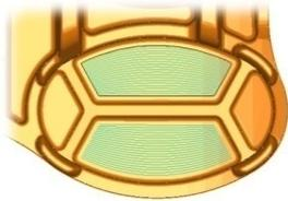
Morph machining allows the user to control a toolpath using flow boundaries and direction profiles. This cavity form is an ideal example of this strategy. Morph machining can be used in conjunction with cutter contact angles.
