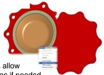
**NCG CAM** also has the ability to create internal fillets, this can in some instances allow a more flowing toolpath. Planar patches can also be created to cap or protect areas if needed.
