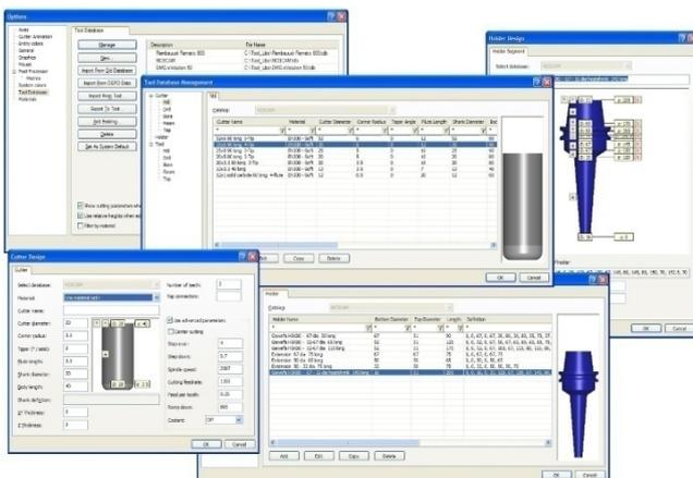
**NCG CAM** can store a wide range of tool-holders and cutting tools in separate libraries, so the users can set-up a range of holders which are suitable for use with the cutting tool. Both the cutting tools and holders can be created graphically and then stored in the relevant library. These libraries can be specified and named for individual machine tools or materials, and set-up to have tool numbers, spindle speeds, rapid feed, ramp feed, cutting feed and coolant or air blast options.
