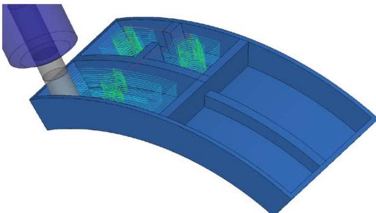
Multi-Surface Roughing of pockets with doubly-curved surfaces, offsetting from the top (ceiling) face to the bottom (floor) face using Area Clearance type machining strategies in full 5-axis.
