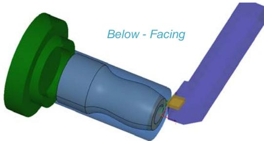
Facing can be achieved using predefined Stock or using the finished part with pass extensions. There are options available for Rough facing using multiple passes or Finish facing in one pass.
