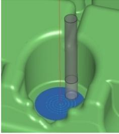
This creates an archimedean spiral toolpath from a given focal point, generating a constant contact as it machines within a given boundary. It is ideally suited for use on round shallow areas using contact angles between 0° – 30°, in conjunction with the waterline machining for the more vertical faces 30° – 90°. These passes can be constrained to a boundary or by the selected surfaces.
