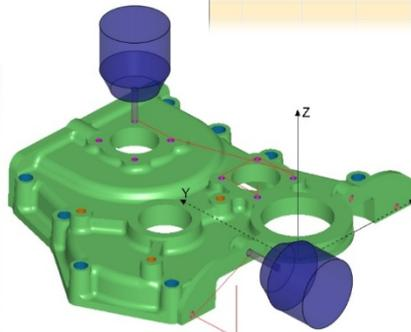
Cycles supported on all post-processors are: spot drilling, deep drilling, deep drilling with chip break, reaming, tapping left and right hand, thread milling (internal, external, left hand and right hand), boring, boring with spindle orientation and bore milling.
