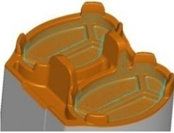
The constant offset machining strategy is used for maintaining a constant equidistant step-over from one tool pass to the next, irrespective of the slope angle of the part. This can also be used in conjunction with cutter contact angles, within any boundary or applied to the whole part.
