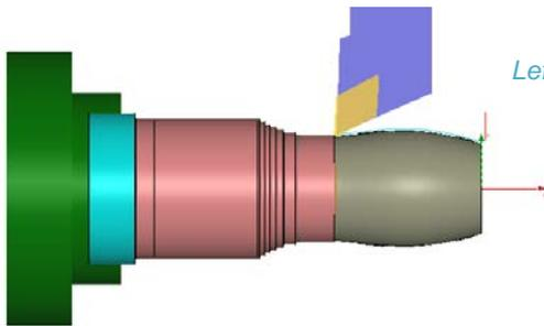
Finish Profiling also includes Undercut protection to avoid Tool Holder collision on the trailing edge whilst turning.
