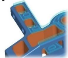
Should the user require to machine these flat areas with more than one pass, the passes can be axially (along the tool axis) offset by a user any number of times.
