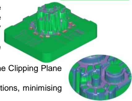
**Waterline ( Z –Level ) Machining Using Surface Contact Angles**
