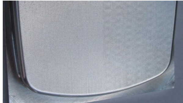
Above – Machined part . Left - True surface machining. Right - Machining triangulations.
