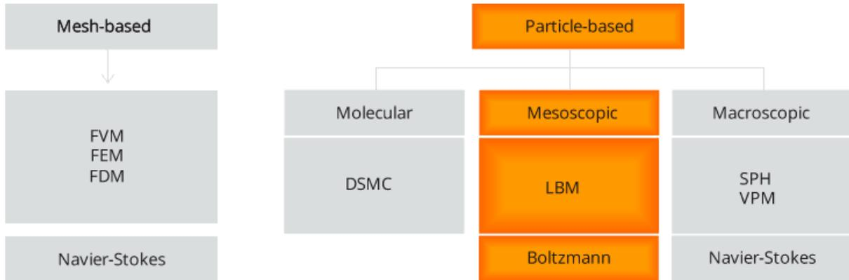
The discretization approach in XFlow avoids the classic domain meshing process and the surface complexity is not a limiting factor anymore. The user can easily control the level of detail of the underlying lattice with a small set of parameters, the lattice is tolerant to the quality of the input geometry, and adapts to the presence of moving parts.
