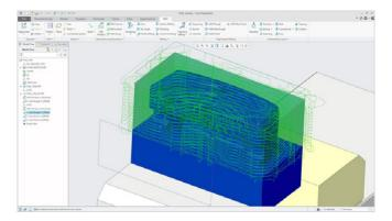
High-speed machining roughing sequence, multi-threaded for fast computation.
