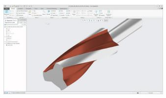
Volume helical sweep – calculate accurate geometry for a Grinding Wheel Scenario.
