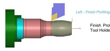
Finish Profiling also includes Undercut protection to avoid Tool Holder collision on the trailing edge whilst turning.
