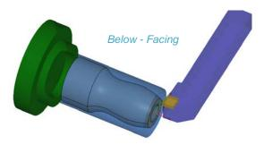
Facing can be achieved using predefined Stock or using the finished part with pass extensions.
