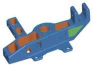
Horizontal area and core horizontal area machining both have similar smoothing characteristics to area clearance and can detect all flat surfaces on a part, with or without using boundaries.
