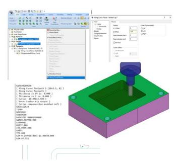
The optional pass overlap allows the cutter to overlap the starting position (closed profiles) to help reduce a 'tool line', giving a better surface finish.
